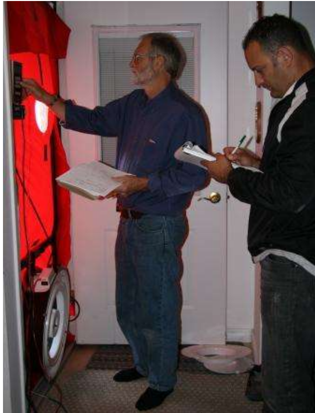
Certified Energy Advisor Stephen Fancott, left, and Steve Goldberg, who conducts quality assurance of AEA advisors for Natural Resources Canada, use a door blower to test the air tightness of a Yellowknife home.
