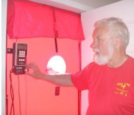
Certified Energy Advisor Steve Outlet of the Arctic Energy Alliance conducts a blower door test to determine the air tightness of a home as part of a Home Energy Evaluation in Tsiigehtchic.
